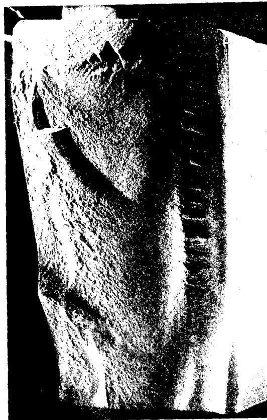
Figure 45. Fracture Surfaces of Hot Pressed Silicon Nitride Specimen 4-6, Showing Corner Fracture Initiation Site.
