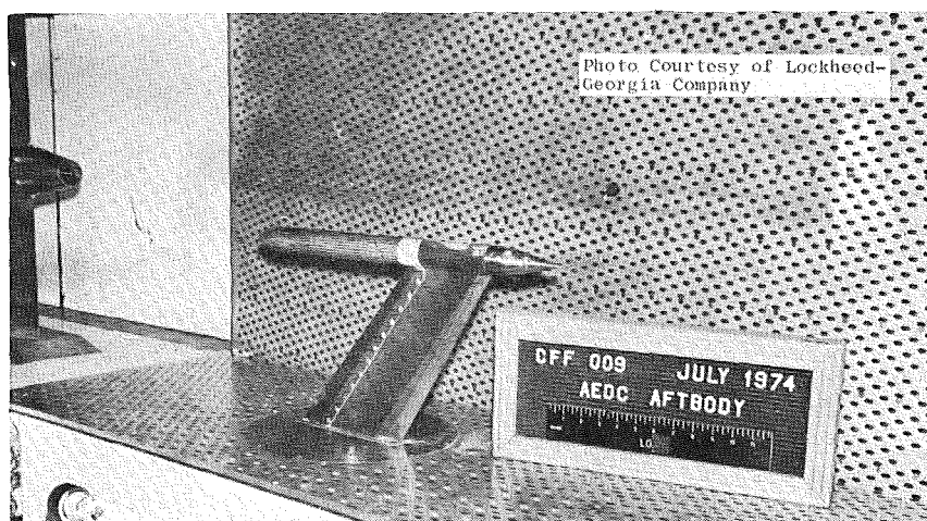
Figure 2. 0.15-scale model installed in the Lockheed-Georgia CFF, Phase II.
