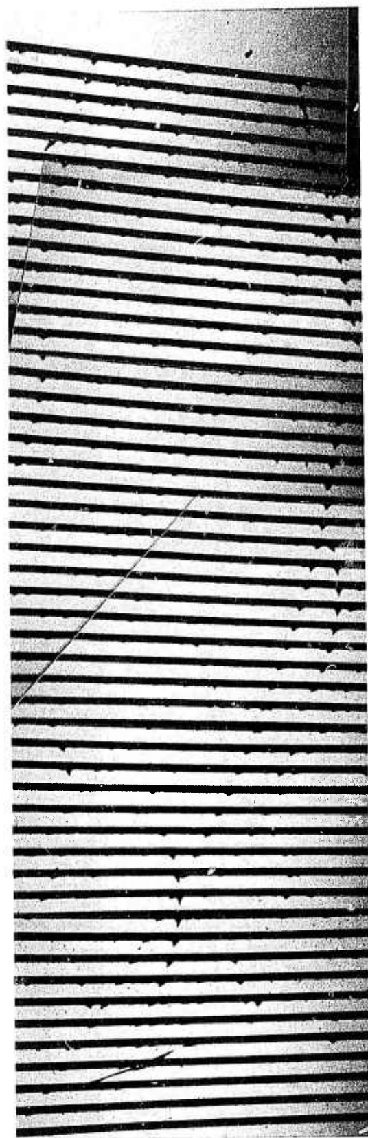
Figure 32 Polishing Damage in a Field of Etched \text{LiNbO}_3 Waveguides. Lower photograph at \sim 100\text{X} . Upper left- and right-hand photographs at \sim 250\text{X} and \sim 500\text{X} , respectively.
