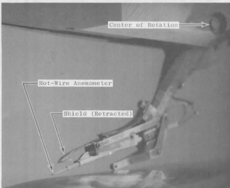
b. Hot-wire anemometer probe, mechanically actuated shield Figure 3. Concluded.
