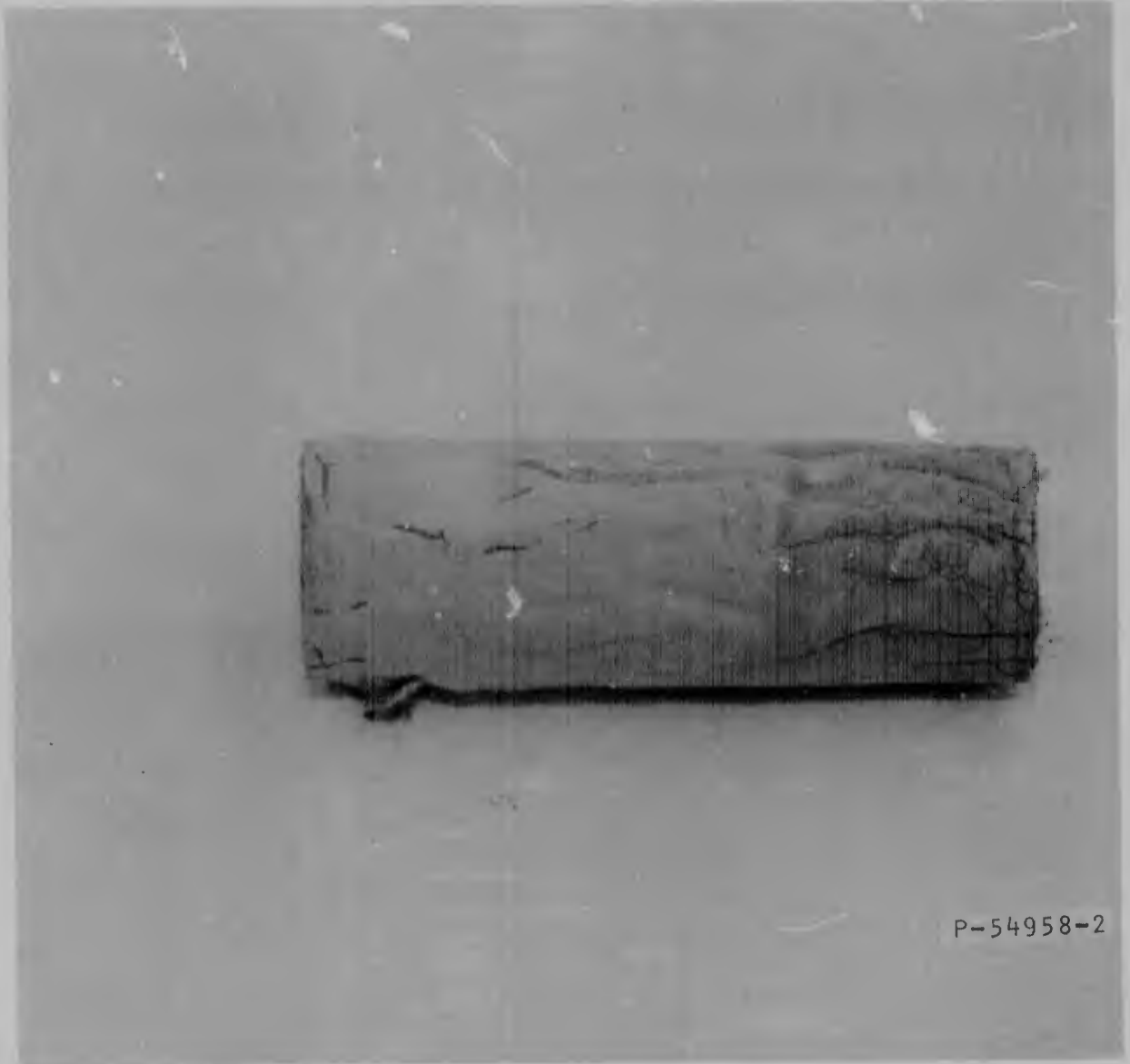
FIGURE 55 VIEW OF BALSTON COALESCER ELEMENT AFTER TEST
