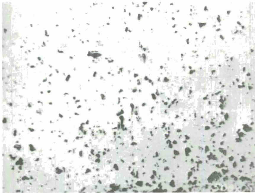
FIGURE 4 Cross-section of deposit that appeared to have inclusion of TiO_2 but gave no positive analytical test for Ti. Dark areas are probably oxides of chromium or small voids in the chromium. Original 550X.
