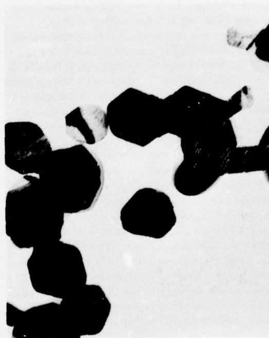
Fig. 4. An example of hexagonal platelets collected from the chamber walls. These hexagons are approximately 130 nm on a side (40,000 \times plus photographic enlargement).
