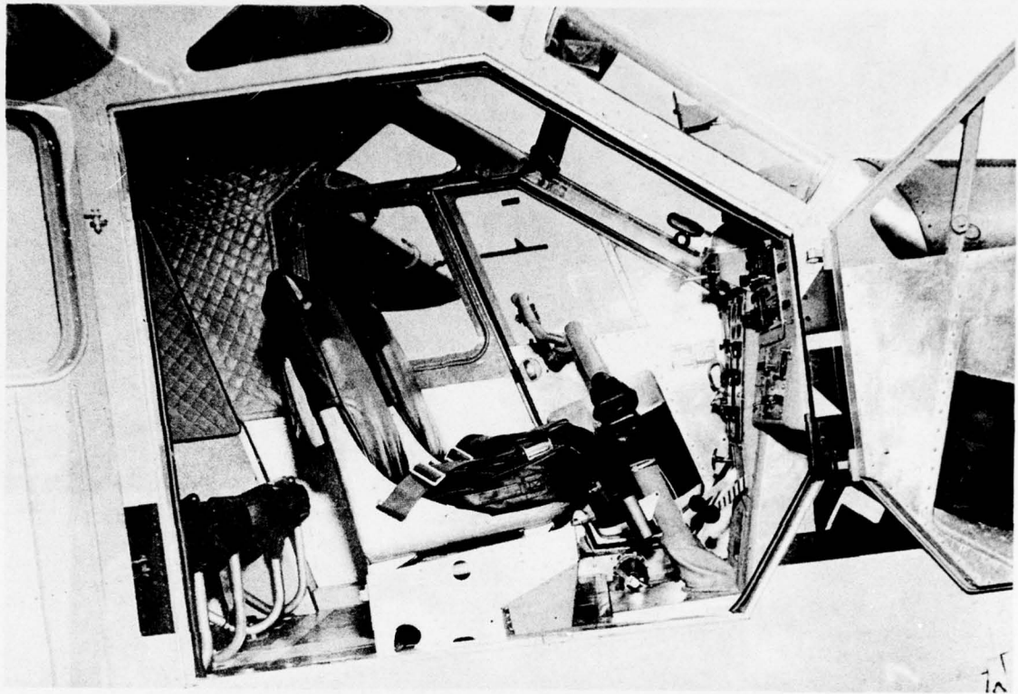
Crew compartment with right double door open. (Note small window over closed left double doors.)
