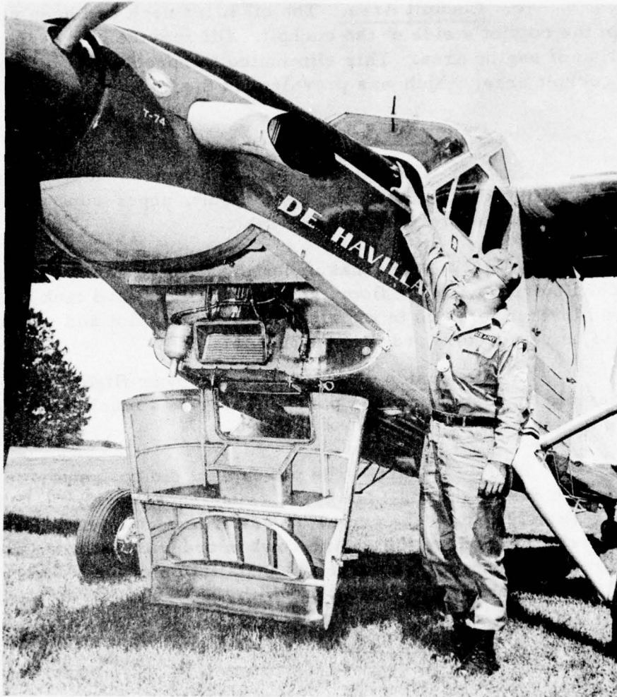
Nose of the Turbo-Beaver with lower engine-access cowling open
