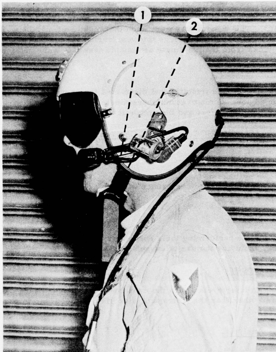
Figure 4. Line of pull of old chin strap (arrow 1) and line of pull of new chin strap (arrow 2).
