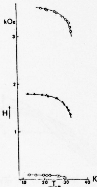
Fig. 208. Transition fields versus temperature for H \parallel c axis of RbCoCl_3 \cdot 2H_2O . After ref. 281.
