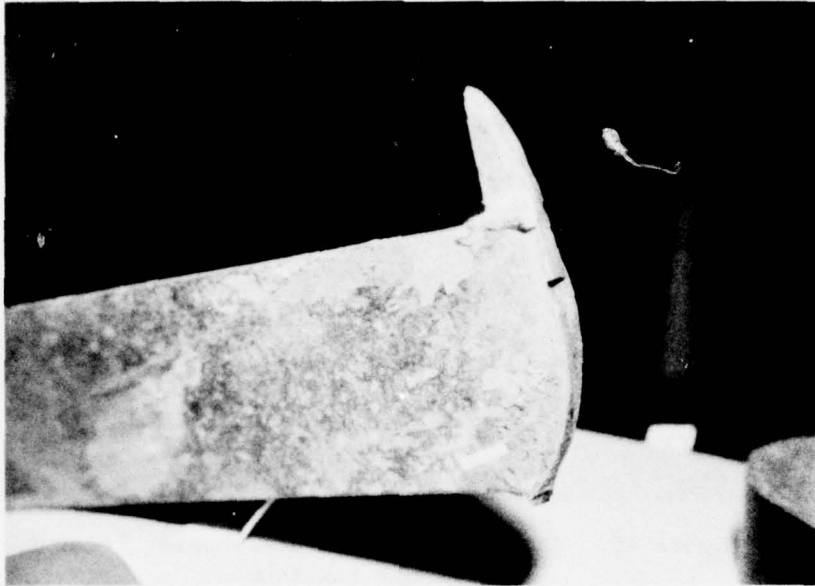
Figure A4. Broken bar showing portion of beam attached
