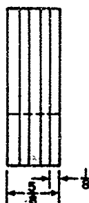
Fig. A2 — Configuration of specimens used for studies of thin-section materials. (Conversion factor: 1 in. = 2.54 cm.)
