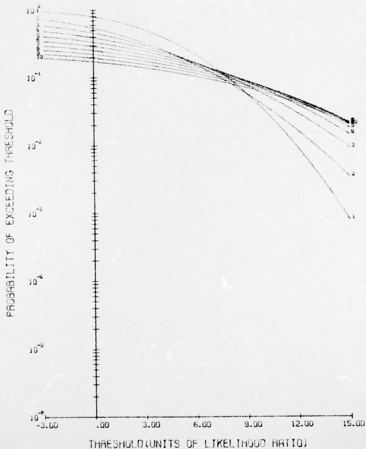
Fig. 21 PROBABILITY OF EXCEEDING THRESHOLD VS THRESHOLD FOR S/N = 10 DB. NEW TRACKS STARTED ON FIRST PING CYCLE. DESIGN S/N = 12 DB. FAC = 1.00 .
