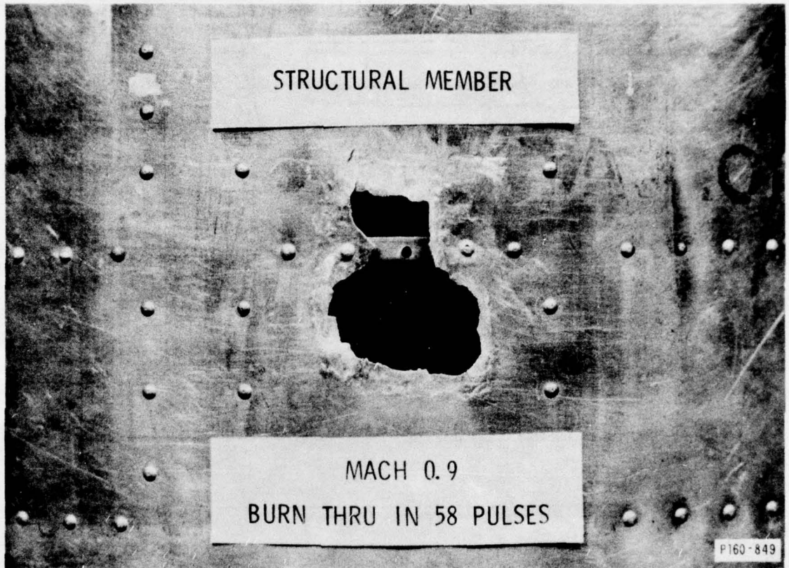
Fig. 11. Damage to structural member produced with Mach 0.9 air flow transverse to surface. The irradiation conditions were the same as given for Figure 10.
