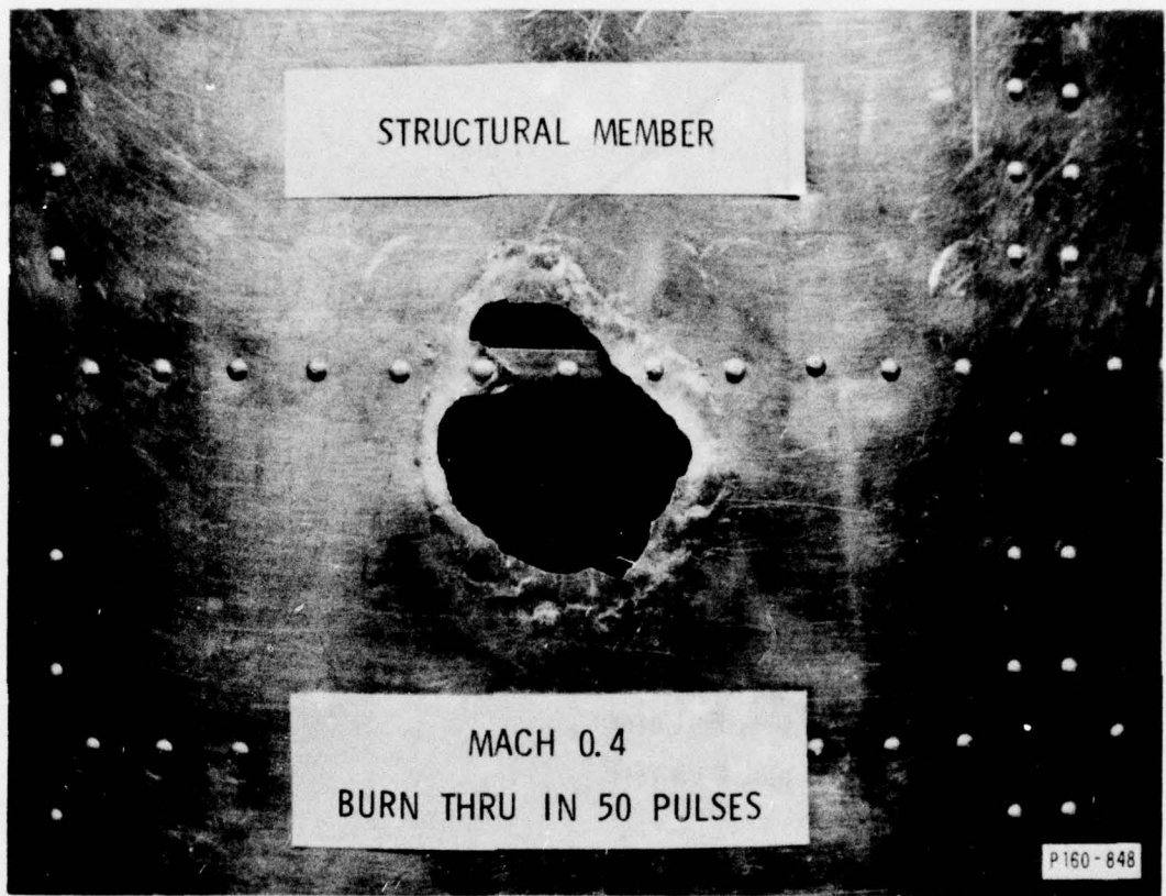
Fig. 10. Damage to structural member produced with Mach 0.4 air flow transverse to surface. The average pulse fluence was \sim 58 \text{ J/cm}^2 and the repetition was 100 pps.
