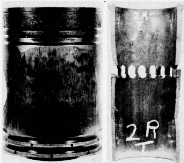
Fig. 14 - 2 Right thrust piston and liner - severe piston and liner scoring, test no. 12, oil code C, NATO F-54 DF, 28 hours.
