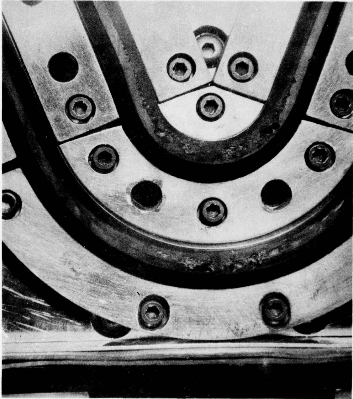
Figure 22 Sliding Seal Set No. 2 - Wear Caused by Repeated Aluminum Bead-on-Plate Welding
