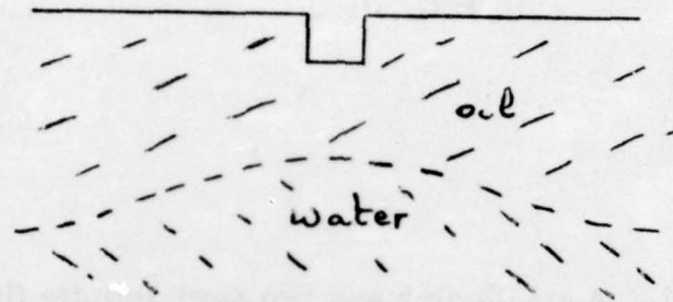
Figure 3: Water cone in vicinity of oil well (based on Karplus [1956, p. 241])
