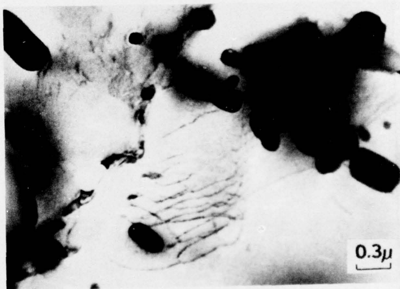
FIGURE 19. TEM OF TiAl + 3% Y 2 O 3 ALLOY T-17.
