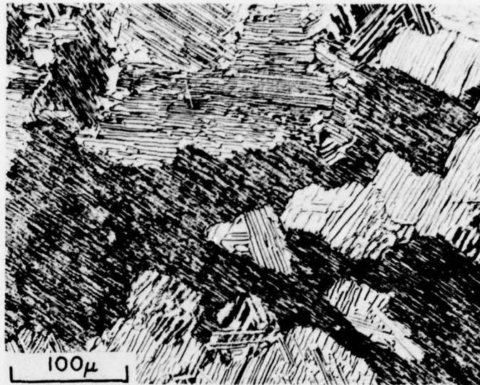
Fig. 23. Alloy 16. Solution treated at 1345°C and aged 24 hours at 800°C, air cool. The coarse mixture of \alpha_2 and \gamma phases was unaltered by aging treatment.
