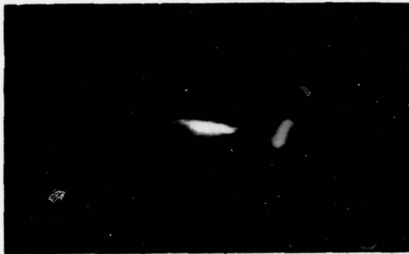
Figure 14. Near field photograph of laser diode light emission.
