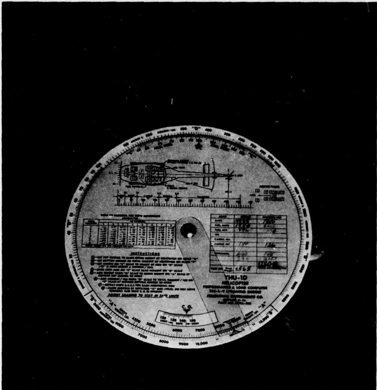
Figure 3. View of the side of the circular computer used to determine center-of-gravity location.
