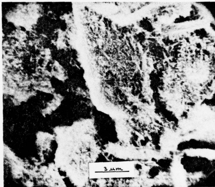
Figure 69 - Active material, 10 cycle PbCa positive plate operated in the trickle discharge routine, plate is fully charged. Substructure of active material showing spiny crystals and some pebbly grains, 5700x.
