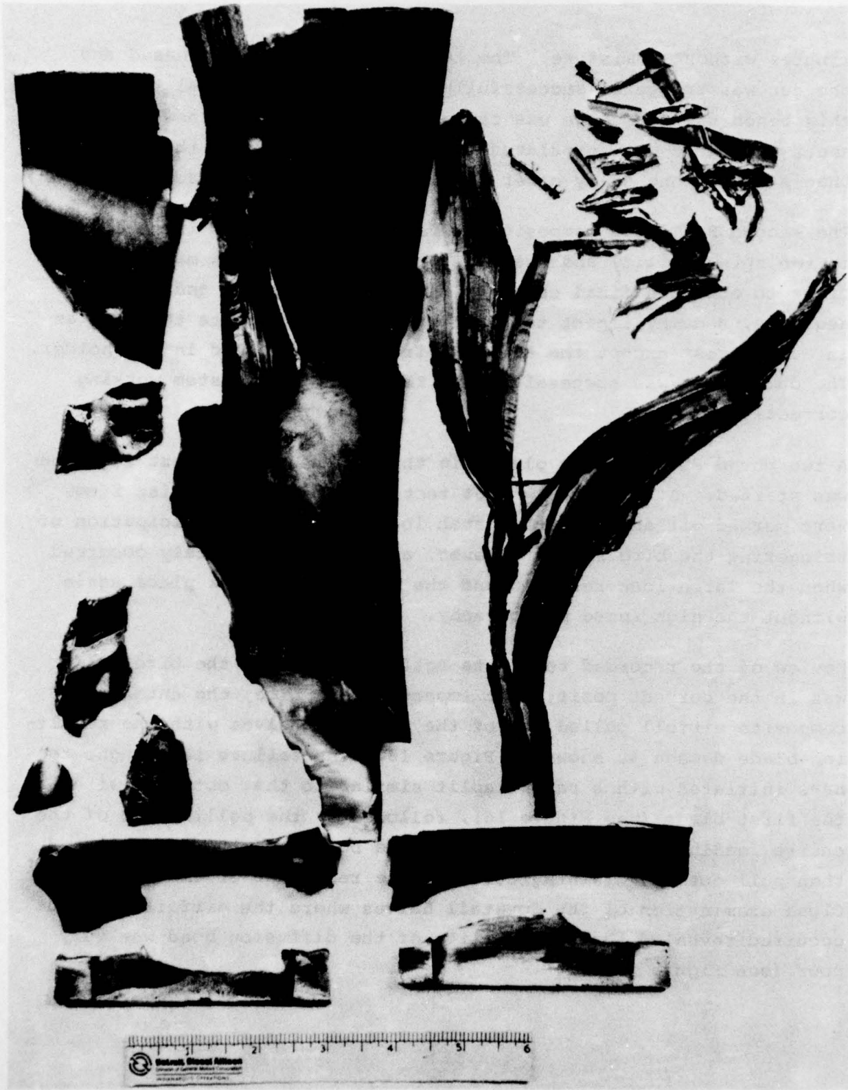
Figure 18. S/N E23C-3 Be/Ti Blade after 2 lb. impact
