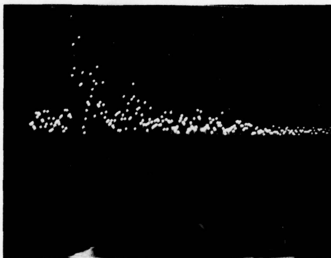
Figure C-5: Fish noise combined with the submarine in Figure C-3 from the HP tape recorder. The output level from the tape had to be reduced in order to avoid amplitude distortion. Thus the submarine cannot be seen.
