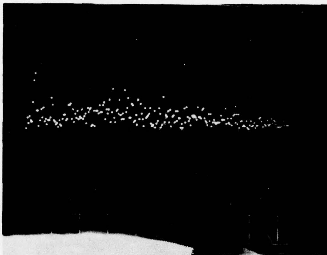
Figure C-4: The same submarine as in Figure C-3, recorded on audio quality tape recorder at 7 1/2 ips. Note the increase in noise level.
