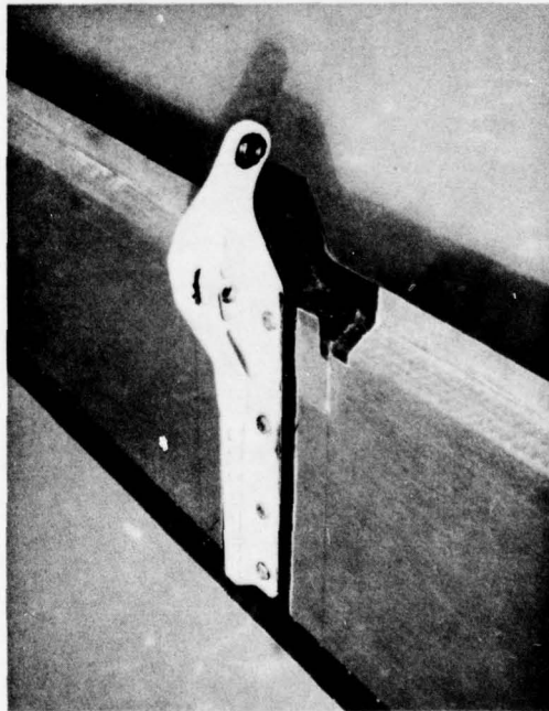
FIGURE 48: INBOARD HINGE ASSEMBLY INSTALLATION,
