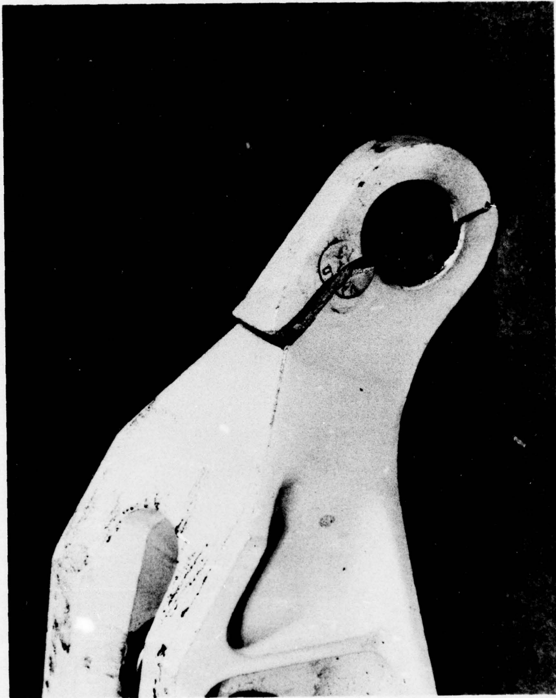
FIGURE B-17 SPOILER NO. 4 --- OUTBOARD FITTING FAILURE
