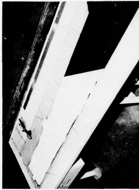
FIGURE 33: LOWER SKIN, LAY-UP OF PLY NO. 6
