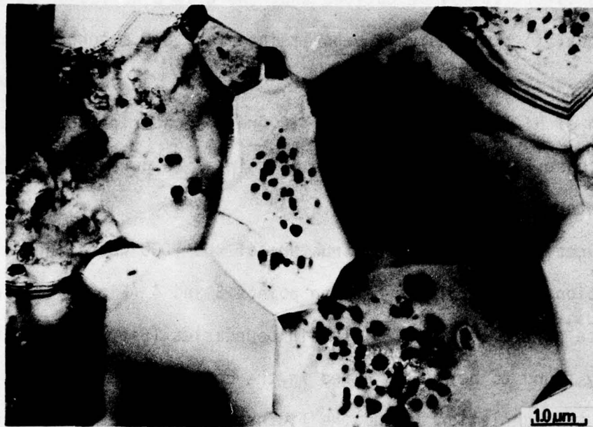
Figure 2 - Structure of a "ARE" Ti-10 % Ni-C coating in a longitudinal section. The coating was deposited at a 1000°C.
