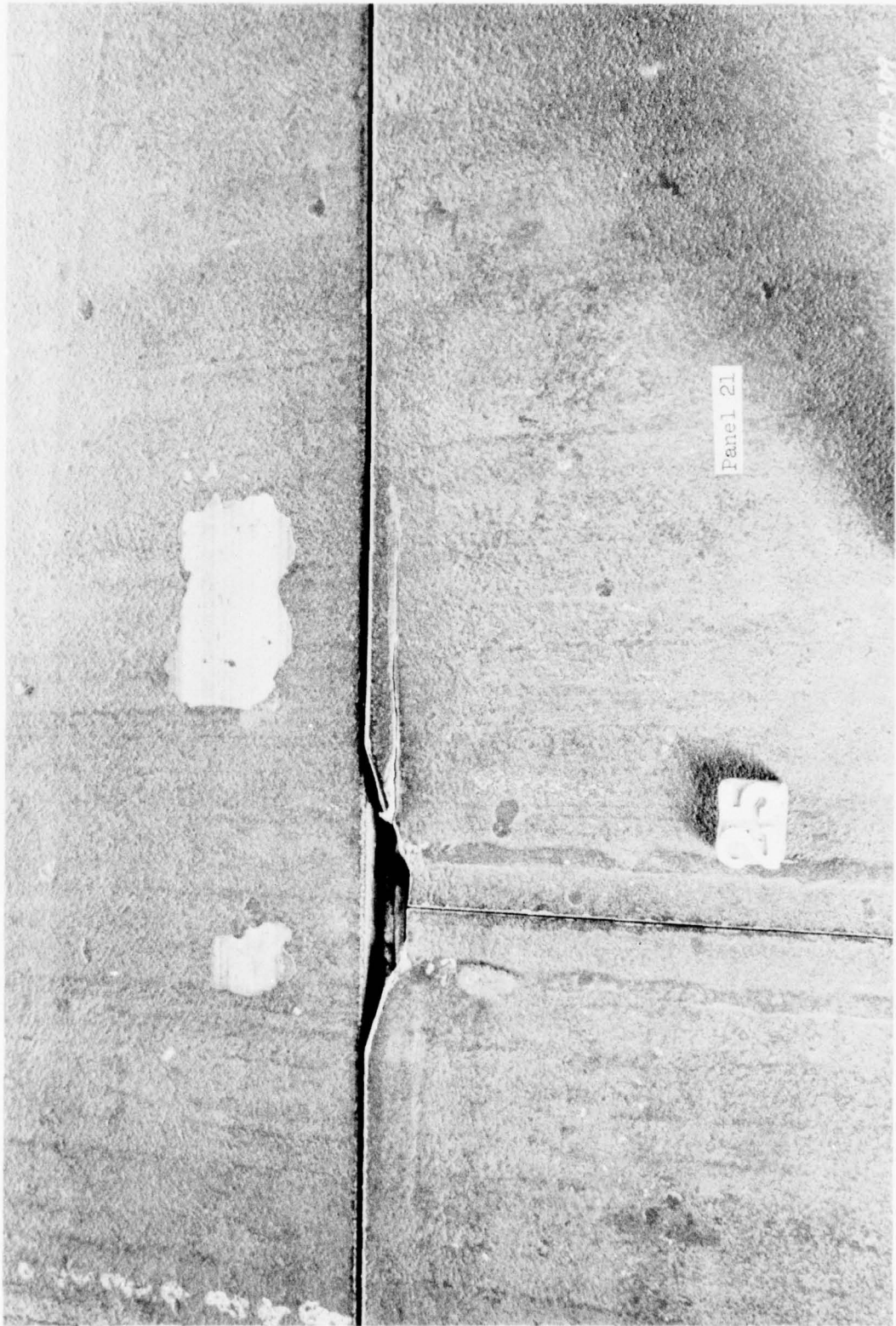
Split in female connector of panel 21 after 1040 coverages, Phase 1
