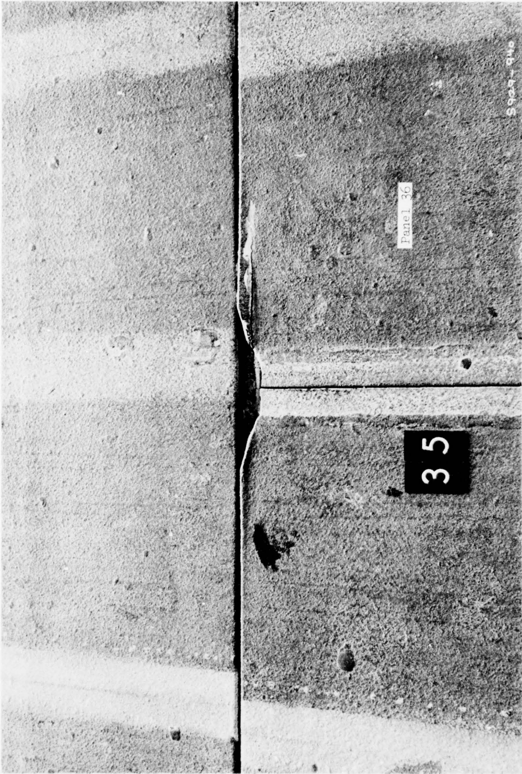
Split in the female connector of panel 36 after 832 coverages, Phase 2
