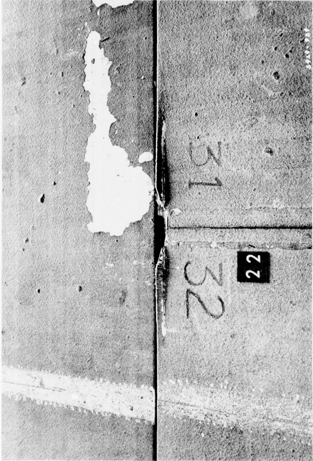
Split in female connector of panels 31 and 32 after 760 coverages, Phase 1
