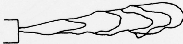
Figure 5: Photographs of the development of spray Ambient density: 16.5 atmospheres, Scale: Nozzle diameter = 0.9 cm.
