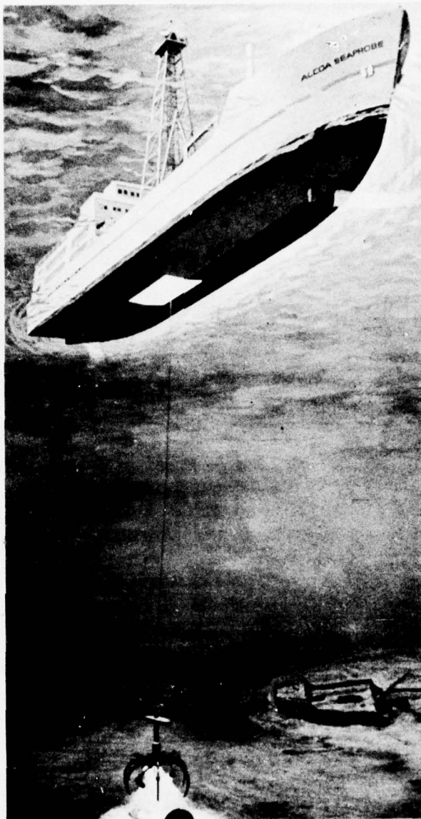
Seaprobe Concept Showing the Cycloidal Propellers, Fore and Aft and the Semi-rigid Drill Pipe String Being Lowered from the Deck Mounted Derrick, Lowered through a Center Well in the Ship's Hull to the Ocean Floor and the Survey Site.
