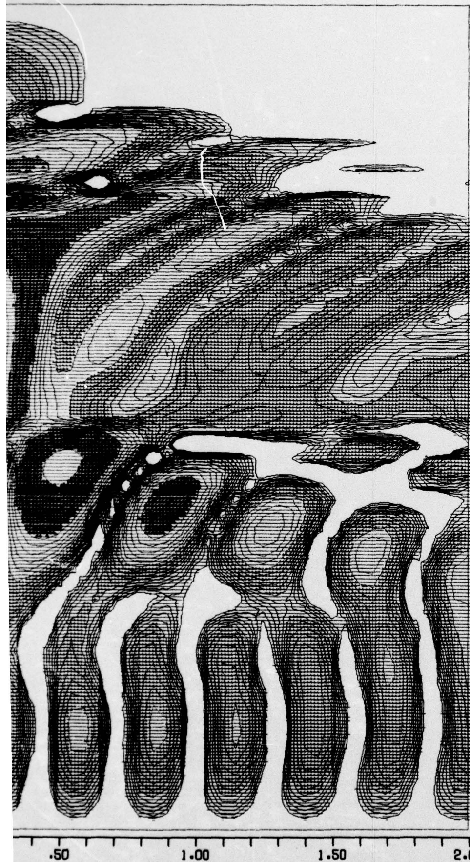
FIGURE 5-11 TIME - ANGLE BEAM PATTERN CONTOUR MAP FOR MODIFIED TRIANGULAR ENVELOPE, PHASE CODED PULSE
