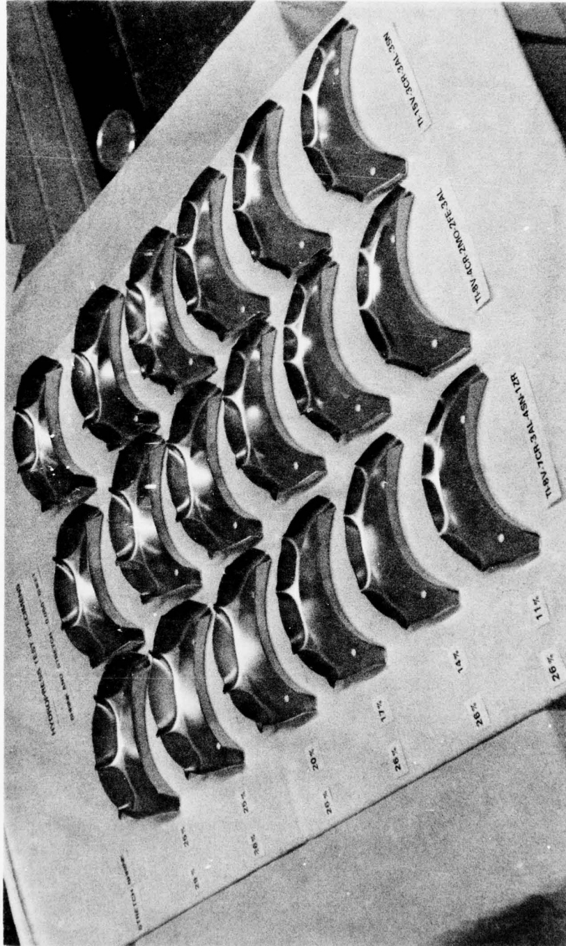
10315 FIGURE 13. HYDROPREC'S FORMED SAMPLES (3" PART RADIUS) FROM 0.050" SHEET OF THREE BETA TITANIUM ALLOYS (26 AND 29 PERCENT STRETCH FLANGES AND 11-25 PERCENT SHRINK FLANGES, VIEW OF CONCAVE SIDE).
