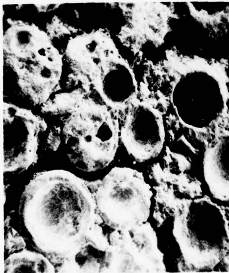
Figure 6 Surface of Specimen Erosion Tested at 3200°F
