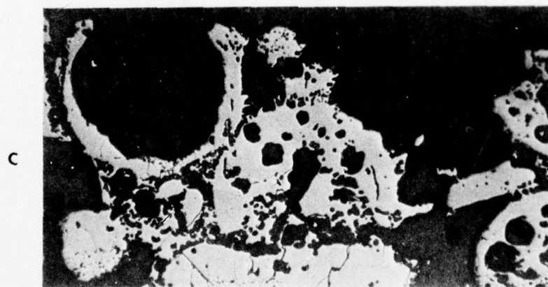
Figure 3 Microsections Near Surface of Post-Test Hot Gas Erosion Specimens: (A) 3000°F, (B) 3100°F, (C) 3200°F (M741383, M74182, M74181)
