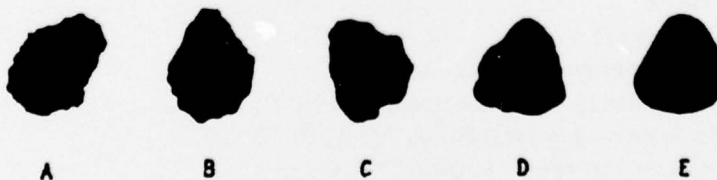
Roundness classes. A: Angular. B: Subangular. C: Subrounded. D: Rounded. E: Well Rounded.
