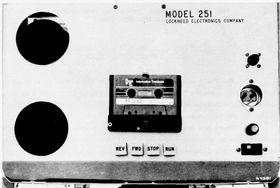
Figure 22. Lockheed Model 251 cassette reproducer
