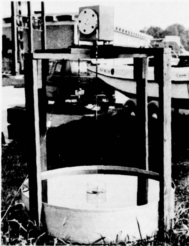
Figure 12. Universal Engineered Systems Model T-66 water-level sensor
