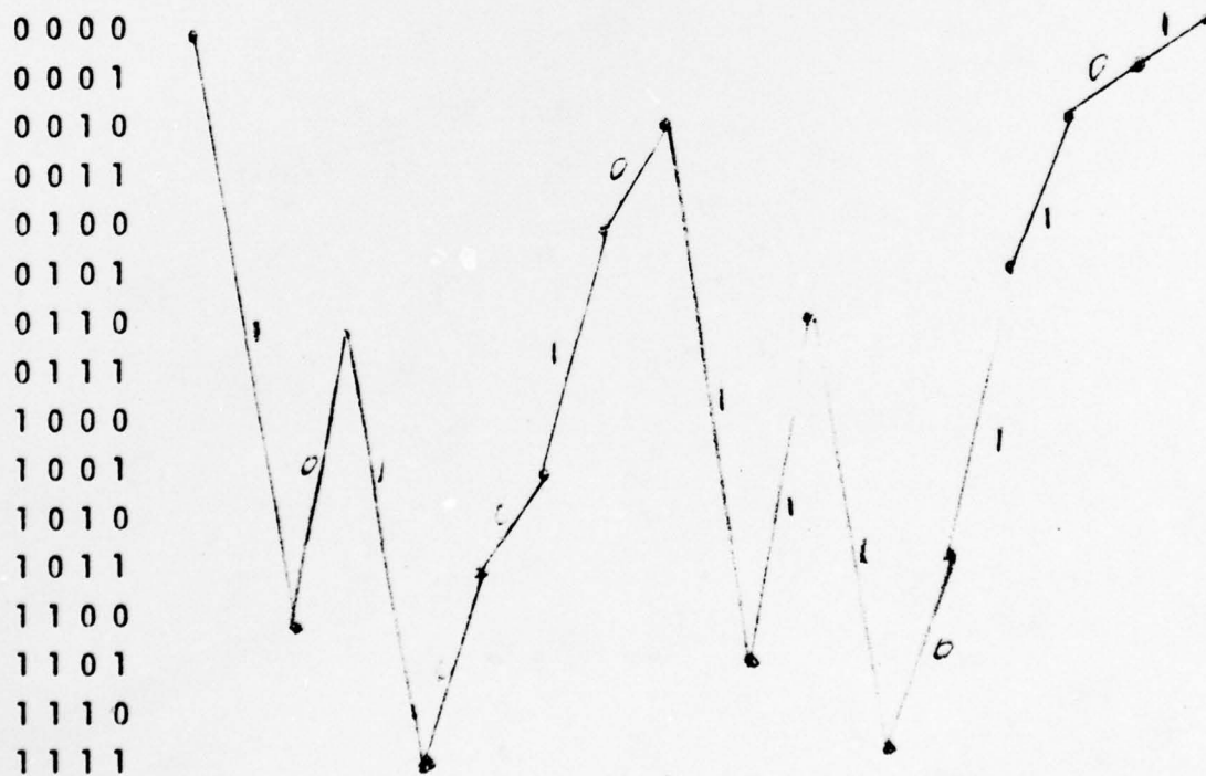
Figure 6. Path in Trellis for Code Word 101001011101101
