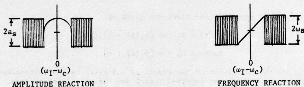
Figure 2. Oscillator reaction patterns as a function of radian difference-frequency between injected and carrier frequencies.
