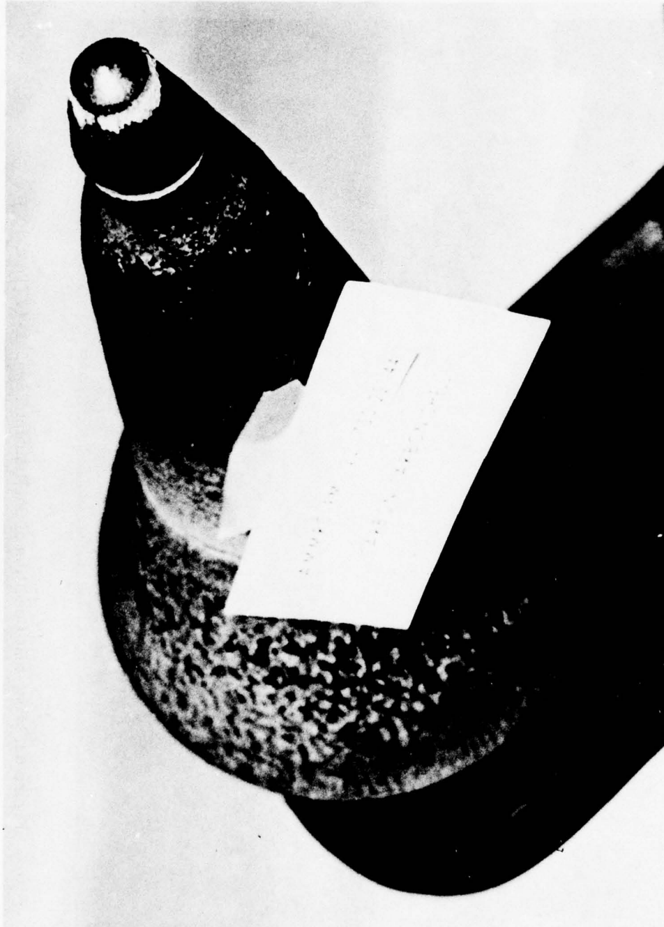
Figure 63: Post-test Surface of Shell Model T50-221-44
