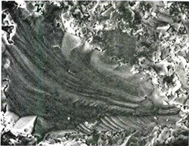
Figure 11. Fracture pattern of hot-pressed Si, indicating large agglomerated grains associated with surrounding small grains as failure origin. The bend bar failed at 8300 psi (MOR). Mag. 700X 19-066-1215/AMC-75
