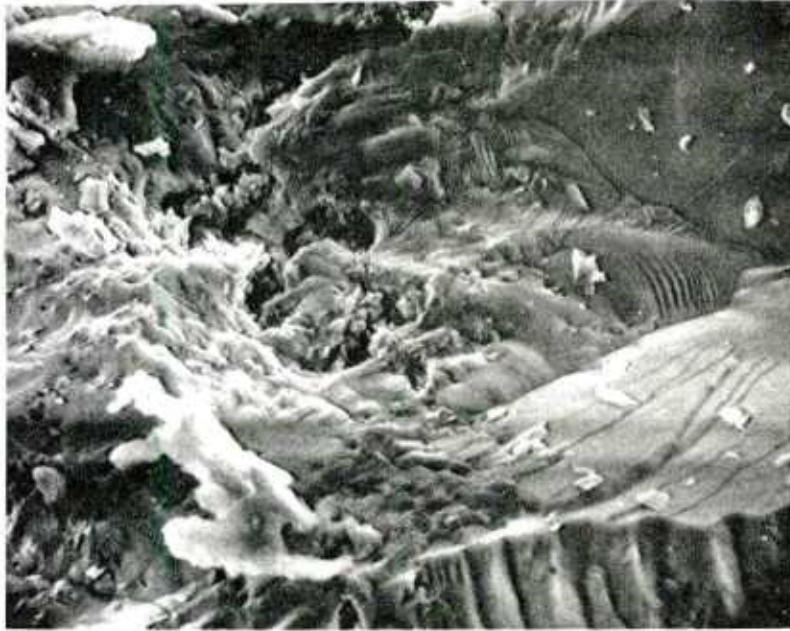
Figure 10. Fracture pattern of Si-20 wt% B 4 C, indicating isolated pore pockets as failure origin. The bend bar failed at 8000 psi (MOR). Mag. 700X 19-066-1215/AMC-75
