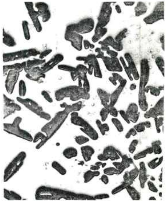
(b) Showing formation of \text{SiC} phase
