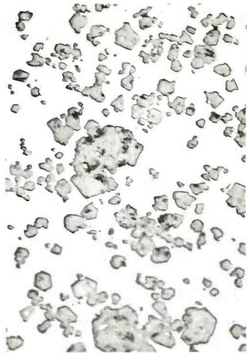
Figure 6. Microstructure of Si-5 wt% C by liquid-phase sintering. Mag. 500X
