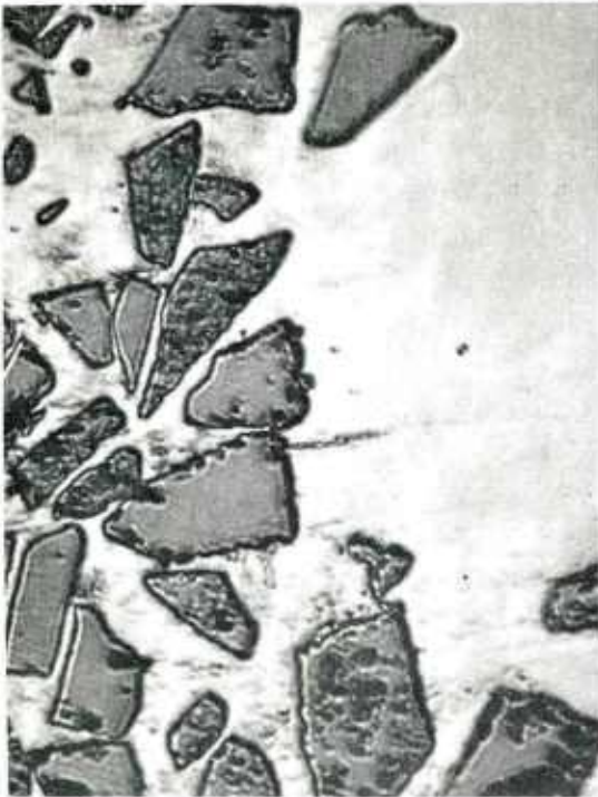
Figure 5. Microstructure of Si-10 wt% SiC by liquid-phase sintering. Mag. 500X
