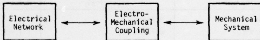
Figure 9. An Electro Mechanical System
