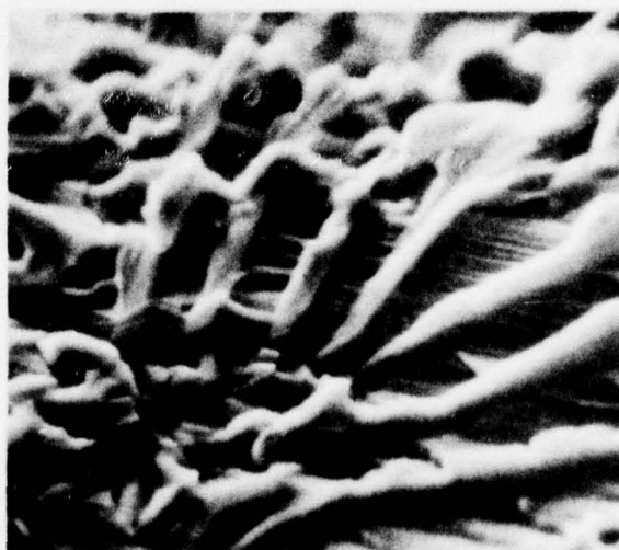
(c) Scanning Electron Micrograph of Fracture Surface Magnification 2000X
