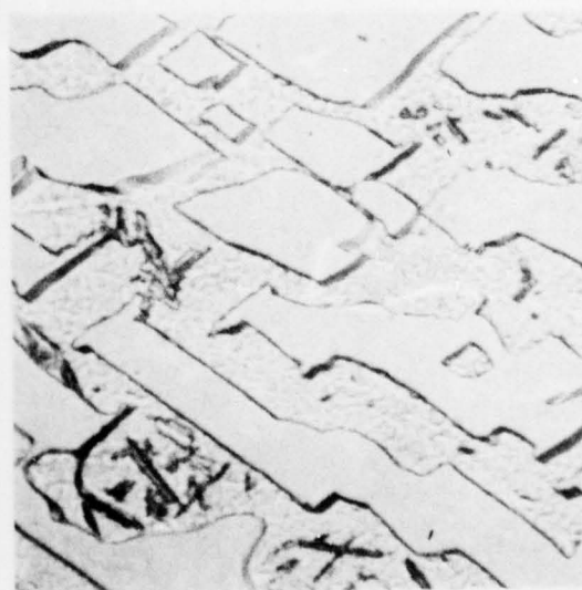
(c) Slow Cool; 3°F/min. Magnification 1000X
