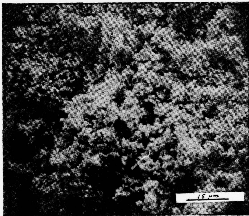
Figure 50. Active material near the grid with little change in its microstructure. Lead-antimony battery 20 cycles, 1280X.
