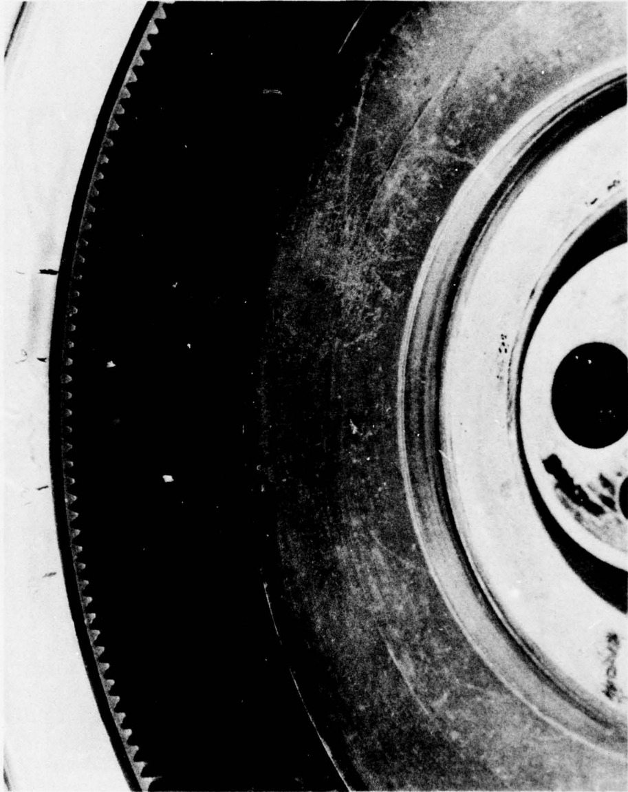
Figure 18. Damage to Teeth No. 1, 6, and 13 of Upper Ground Gear After Run No. 4
