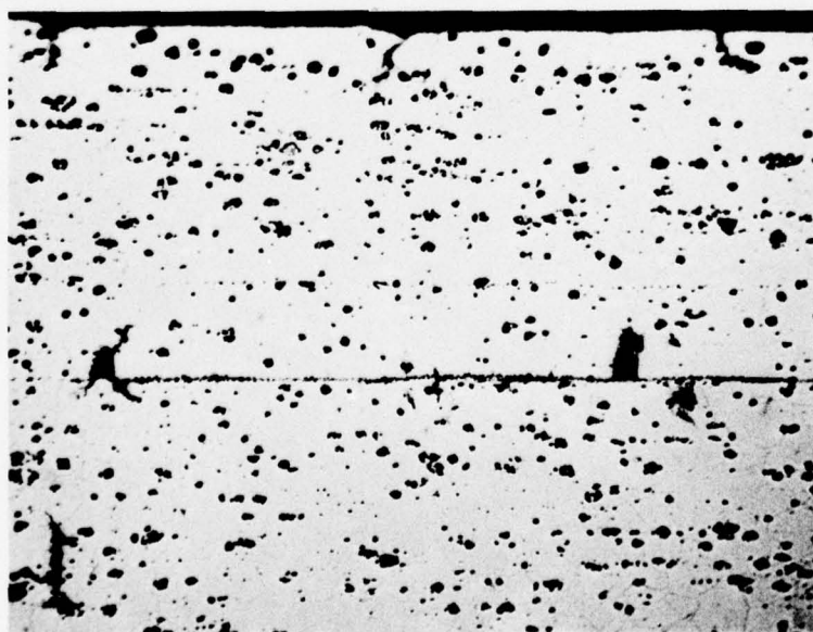
Figure 10. ST+ \gamma' +S+C+F Processed AF2-1DA Alloy Microstructure from Stress Rupture Sample Revealing Grain Boundary Ruptures Originating at Carbide Stringers and the Specimen Surface.
