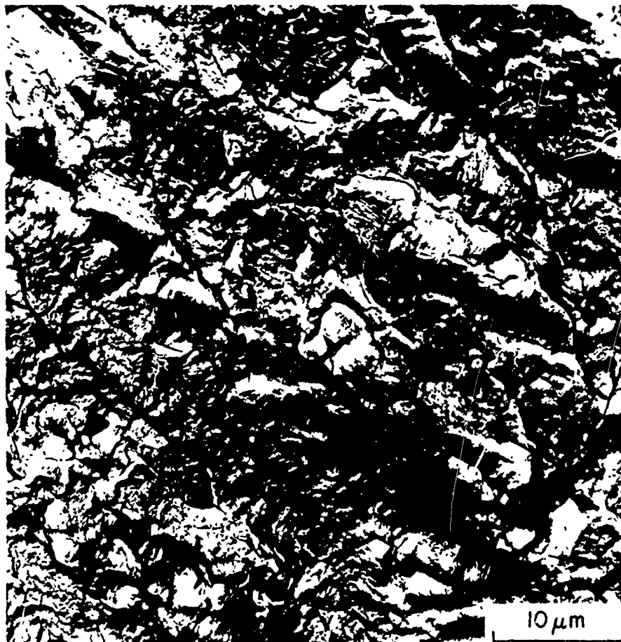
Fig. 8—Cyclic cleavagelike features and striations in the fracture surface for the MA at \Delta K = 17.5 \text{ MPa} \cdot \text{m}^{1/2} . Replica electron fractograph.
