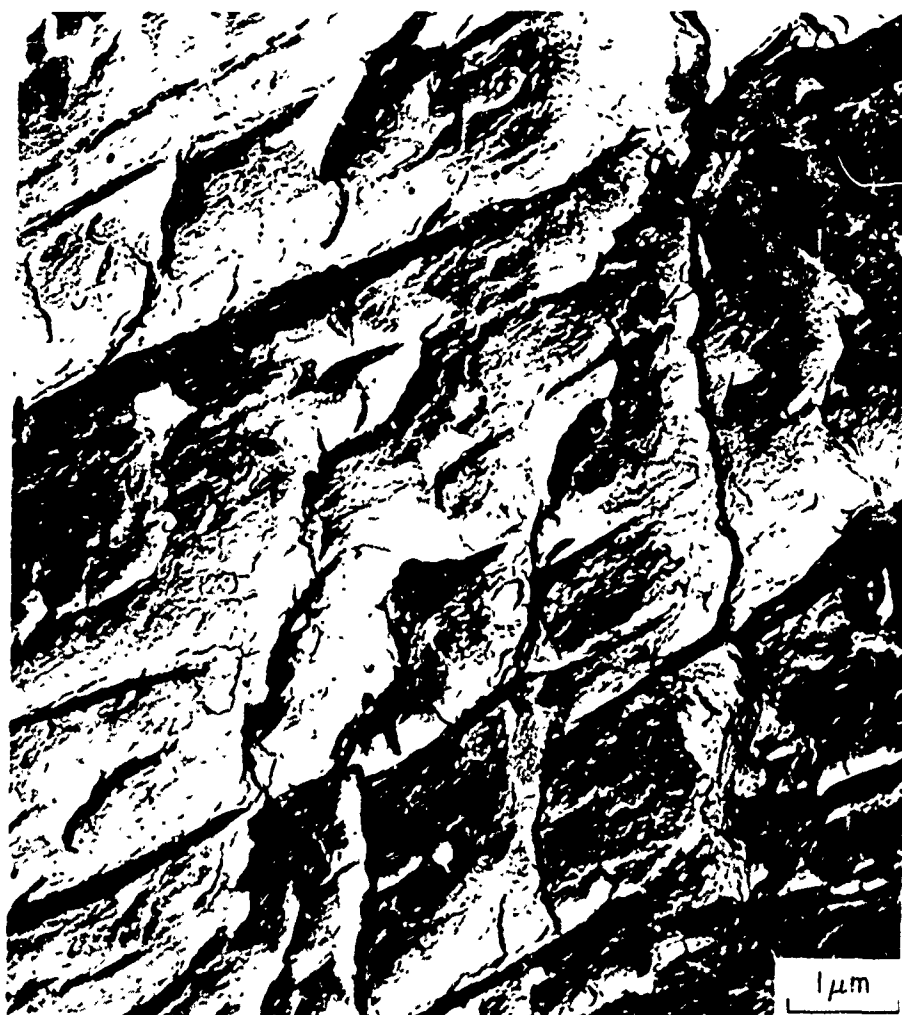
Fig. 10d—Detail of faceted morphology of the BA below T showing fine striations on facet at 14,650X; replica electron fractograph
