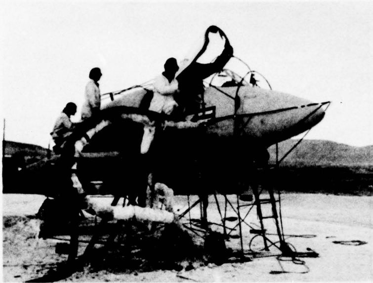
FIGURE E-8. A-4 Enshrouded in Steel Re-Bar Cage for Supporting Exterior Thermocouples. (Neg. LHL 192308)
