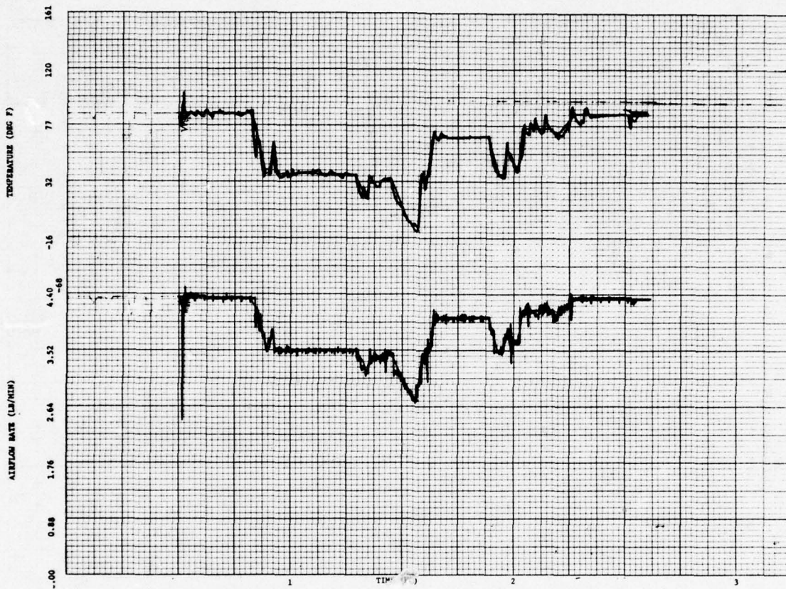
Figure 11. Manual Control of Airflow Rate and Airflow Temperature Profiles
