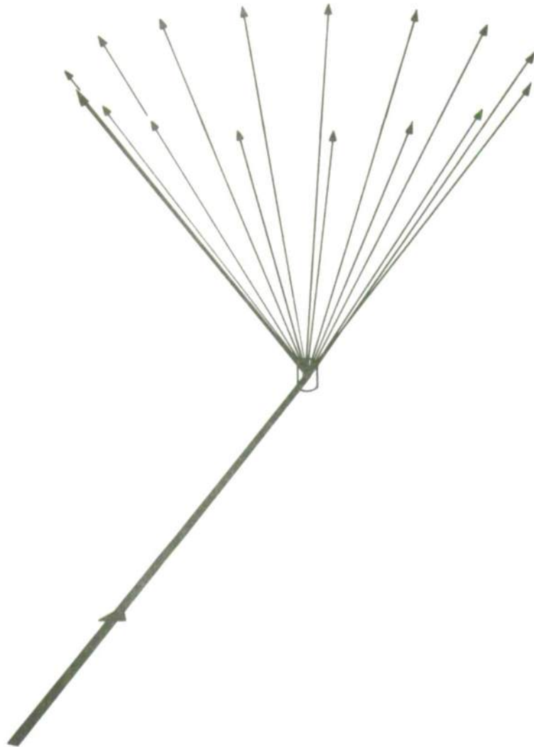
Fig. 7. Specular reflection from a cylinder
