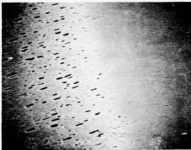
SEM, GaAs, 1000Å, Si 3 N 4 , 750° Anneal (Includes Area Protected by Gold)
