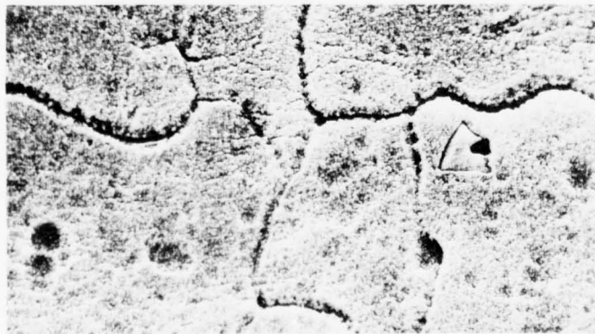
c. VAPOR DEGREASED, ALKALINE CLEANED, DEOXIDIZED, ANODIZED 2,800X
