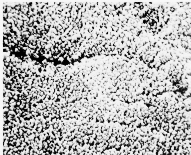
FIGURE A5. CELL STRUCTURE OF STANDARD SURFACE OF BARE 7075-T6 ANODIZED IN PHOSPHORIC ACID
