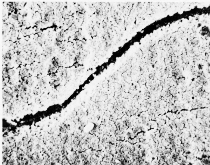
FIGURE A8. SURFACES OF BARE 7075-T6 ANODIZED IN PHOSPHORIC ACID AND REJECTABLE DUE TO INADEQUATE OXIDE CELL STRUCTURE
