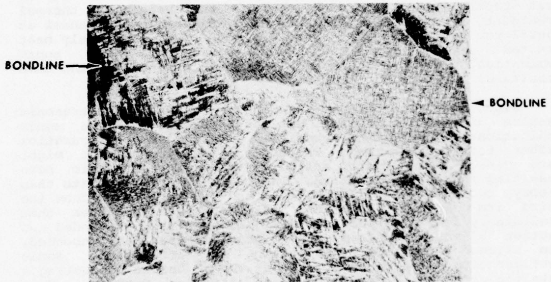
FIGURE 70. MICROSTRUCTURE ACROSS BONDLINE OF THIRD HUB ARM SEGMENT, AFTER FINAL BETA HEAT TREAT AGAIN DISCLOSED NO GROSS LACK OF BOND. 50X
