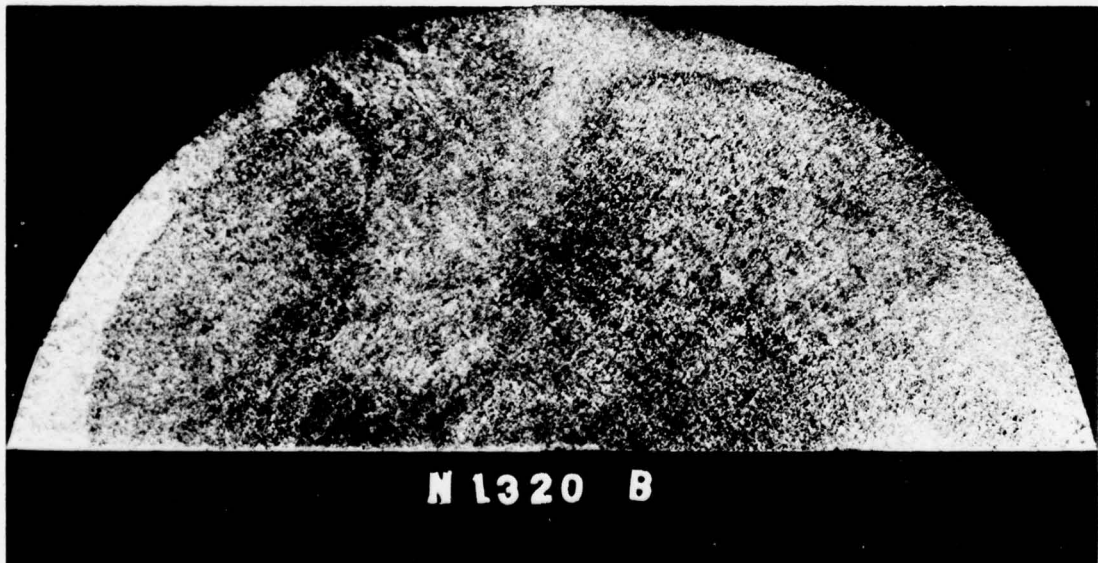
FIGURE 5. MACROSTRUCTURE OF Ti-6Al-4V FORGING STOCK MATERIAL, FORGE-DIFFUSION BOND OF SIMPLE PANCAKE FORGINGS. .75X
