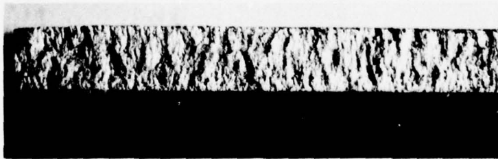
FIGURE 32. IN-LINE SHEAR FRACTURE, TYPICAL STATIC OVERLOAD FRACTURE SURFACE, TRIAL PANCAKE ASSEMBLIES. 4X
