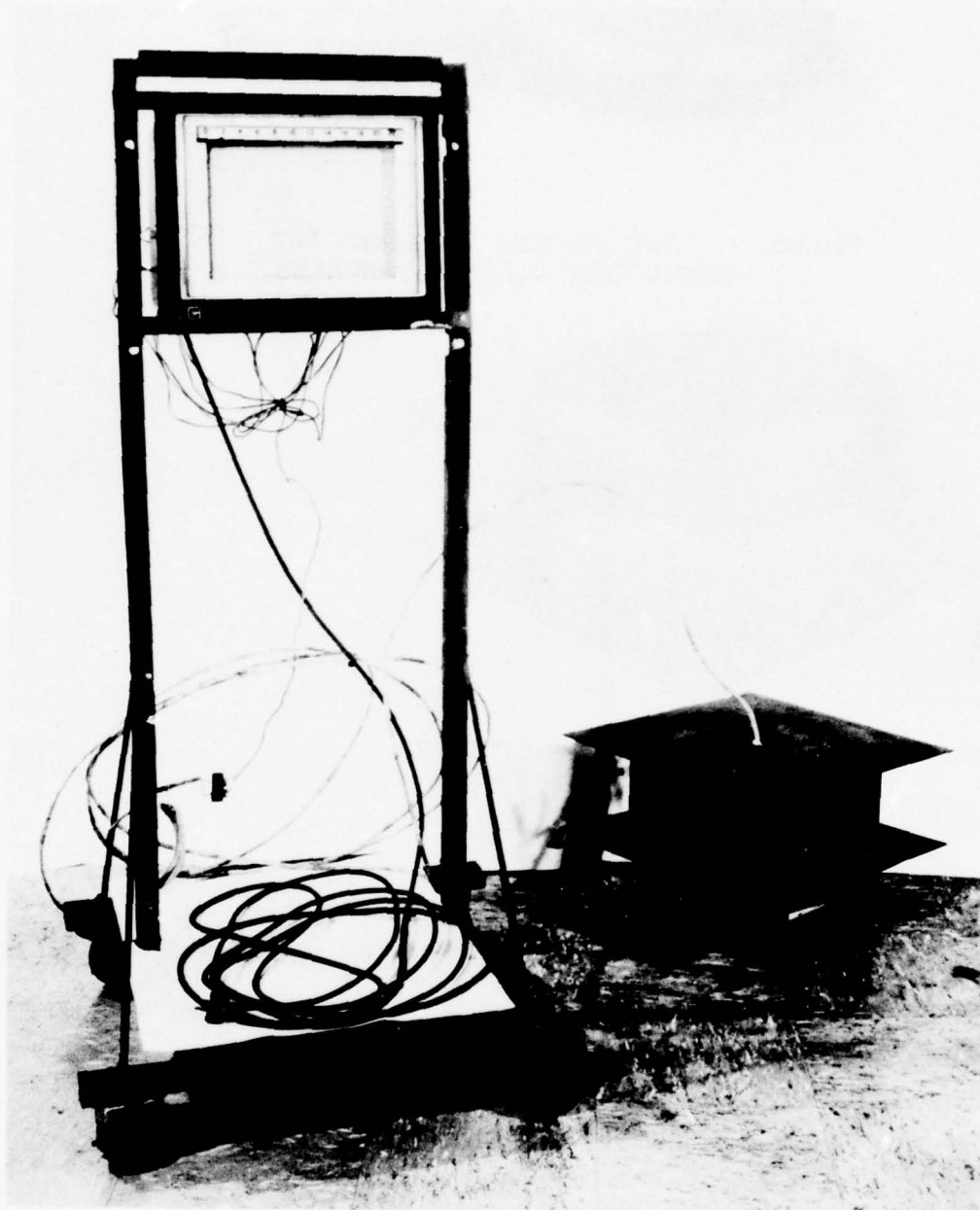
FIGURE 10. TEST RETORT WITH THERMOCOUPLE AND RECORDING INSTRUMENTATION.
