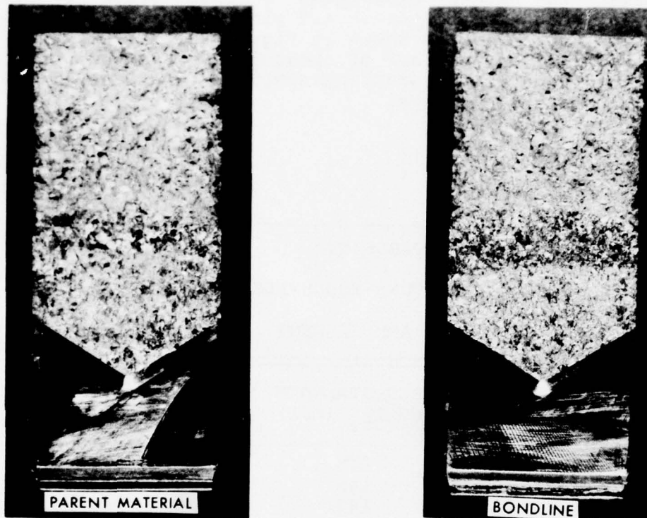
FIGURE 88. FRACTURE TOUGHNESS TYPICAL FRACTURE INTERFACE, HUB ARM SEGMENT. 1.5X
